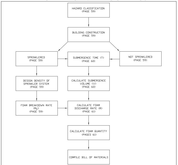
Total Flooding High-Expansion Foam System Flow Chart
