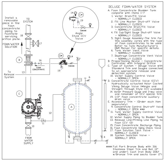
Figure 10: Deluge Bladder Tank Foam-Water System
