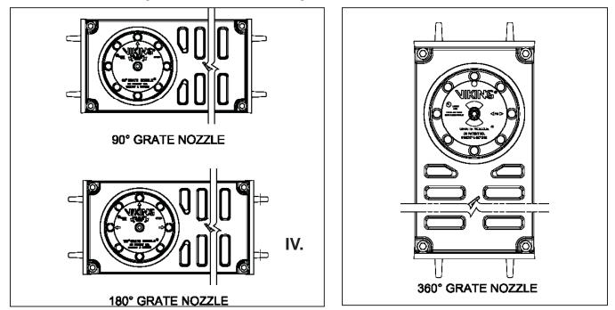
Figure 24: 90° and 180° Grate Nozzles
