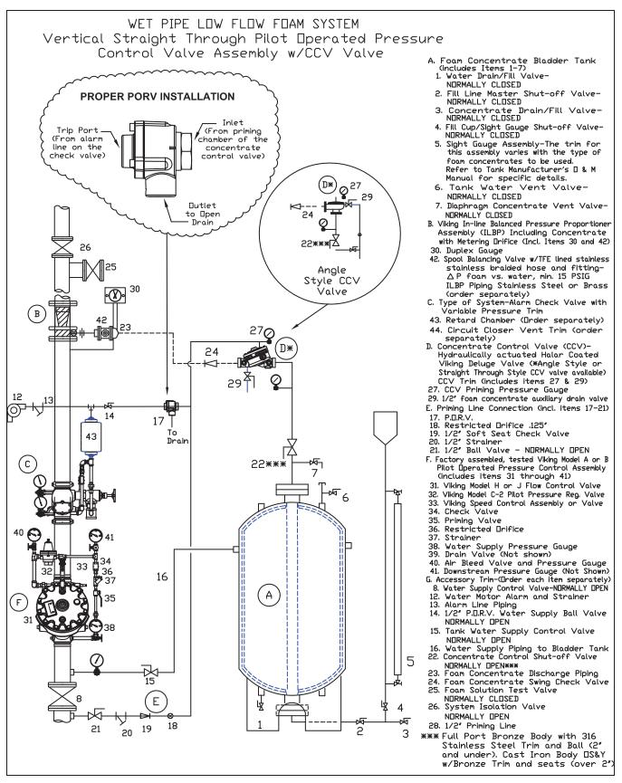
Figure 5: Wet Pipe Low-Flow Foam System Vertical Straight Through Pilot Operated Pressure Control Valve Assembly with Concentrate Control Valve
