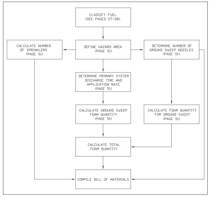
Truck Loading Rack Protection Flow Chart
