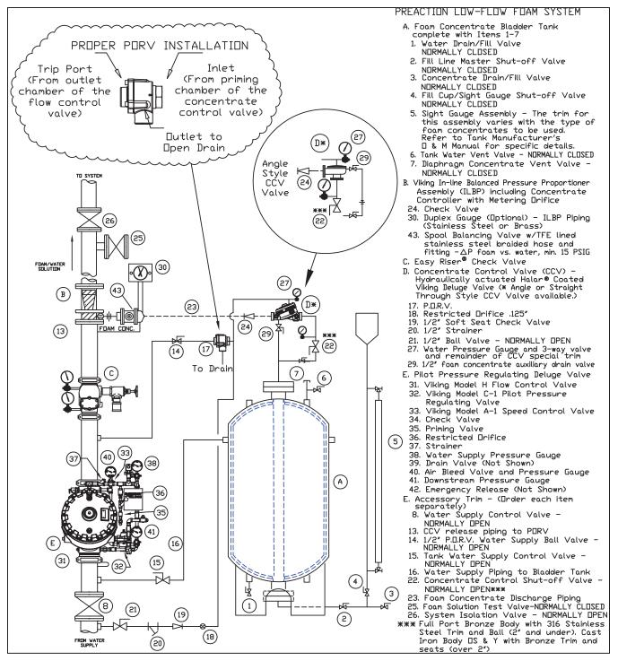
Figure 9: Preaction Low-Flow Foam-Water Proportioning System
