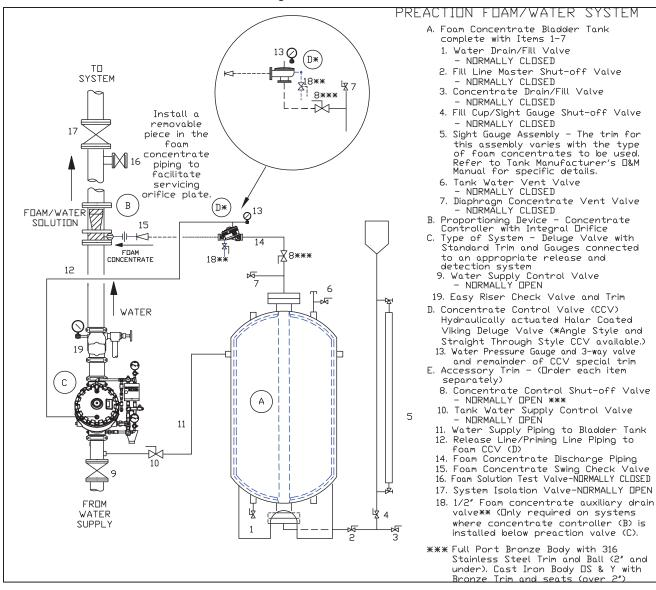
Figure 7: Preaction Bladder Tank Foam-Water System
