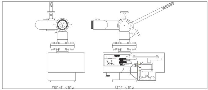
Figure 20: Oscillating Monitor
