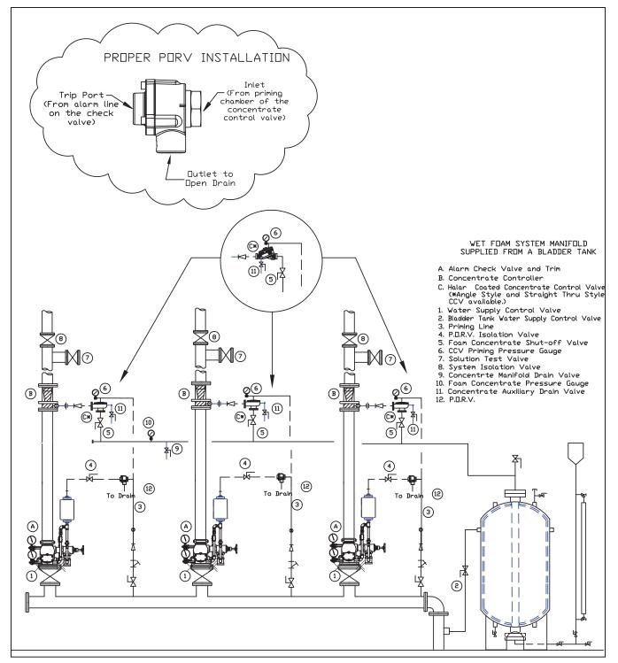
Figure 2: Wet Foam System Manifold Supplied From a Bladder Tank
