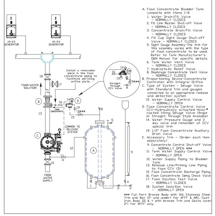
Figure 16: High Expansion Foam System
