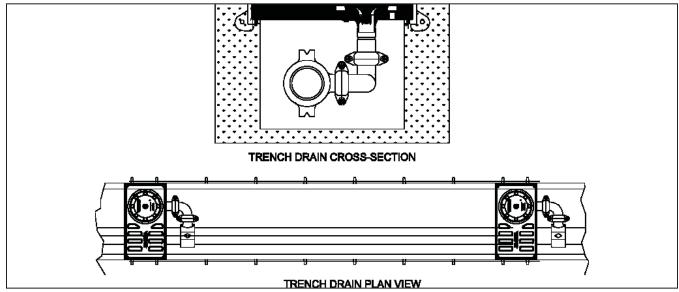
Figure 26: Trench Drains
