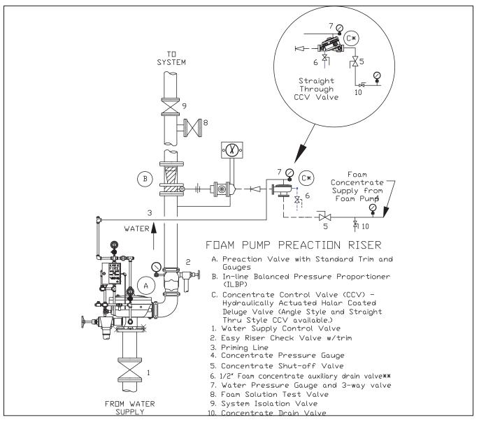
Figure 8: Foam Pump Preaction Riser
