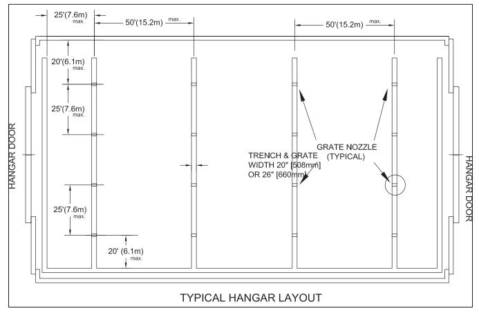
Figure 27: Typical Aircraft Hangar Layout with Grate Nozzles
