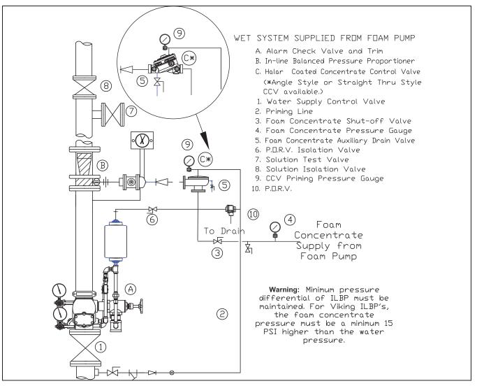
Figure 3: Wet System Supplied From Foam Pump
