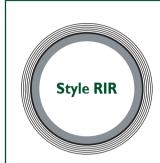
Style RIR fitted with a solid inner metal ring acting as a compression stop, fills the space between flange bore and ID of the gasket. Prevents accumulation of solids, reduces turbulent flow and minimizes erosion at flange faces.
