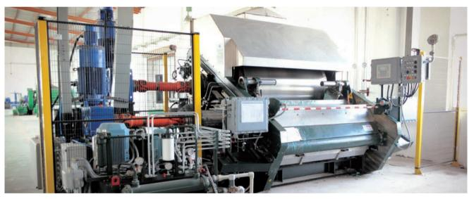
Fully Automatic Compressed Fiber Sheet Manufacturing Line
