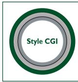
Style CGI, Similar to a CG gasket but fitted with inter ring giving additional compression limitation and providing a heat and corrosion barrier, protecting windings and preventing flange erosion.
