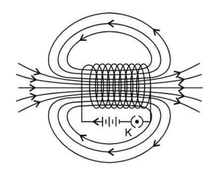
• Magnetic lines produced around a current carrying conductor:
