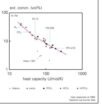
Figure 1: Extinguishing concentration v heat capacity
