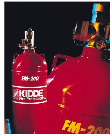
Kidde Fire Protection advises that the maximum fill density for a cylinder of FM-200 pressurised with nitrogen to 360 psi is 1.15 g cm<sup>-3</sup>. Accordingly, the storage capacity for FM-200 is around 1.5 times that of Halon 1301, the closest of all viable replacement agents.
