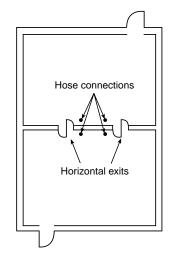
FIGURE A-5-3.2(c) Location of hose connections in exit passageways.
