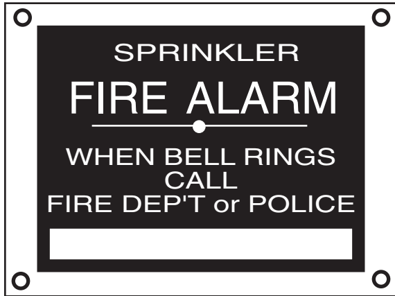
FIGURE A.16.11.2 Identification Sign.
