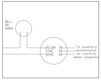
Figure 30: Waterflow Indicator with Two Single-Pole,
