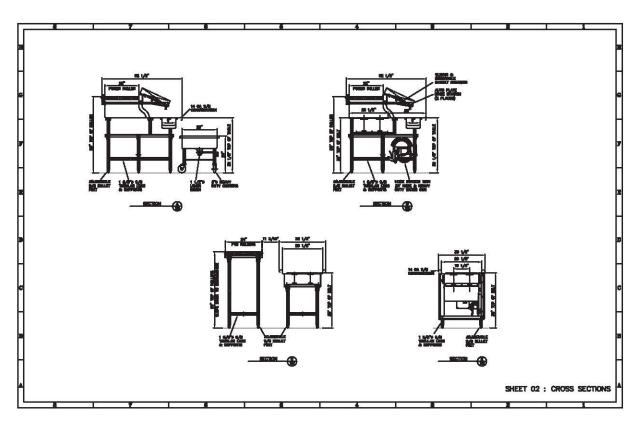
Soiled Tray Handling System: Upracking scrapping system with gravity roller conveyor and dual slat belt conveyor feeding to FT
