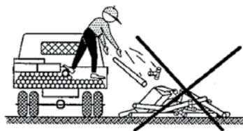
Incorrect way to off-load
