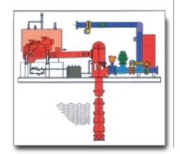
NFPA #20 requires the use of a vertical turbine on systems operating under a static suction lift condition requirement. A-C Fire Pump Systems offers the complete pre-packaged system, pump, driver, controller, low measuring device, control valves, check valves, sensing lines and power distribution panel. This system requires one electrical connection and a water supply.
