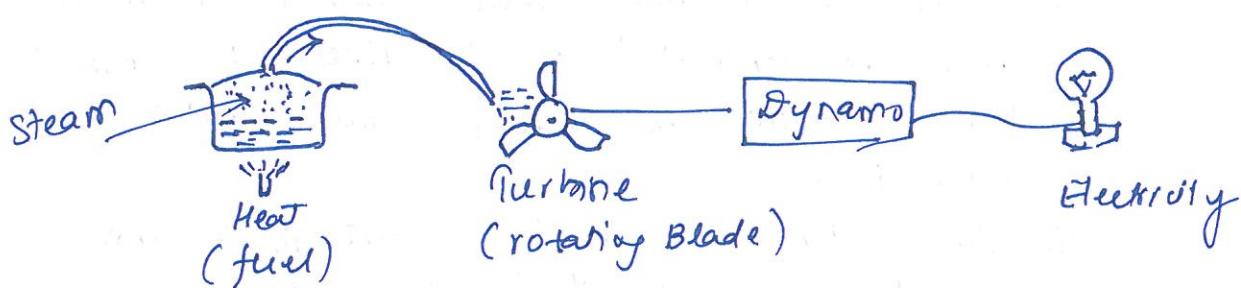
The moving fluid (steam) acts on the blades to spin them and impart energy to the rotor with speed which would turn the shaft of the dynamo and convert the mechanical energy into electrical energy.
