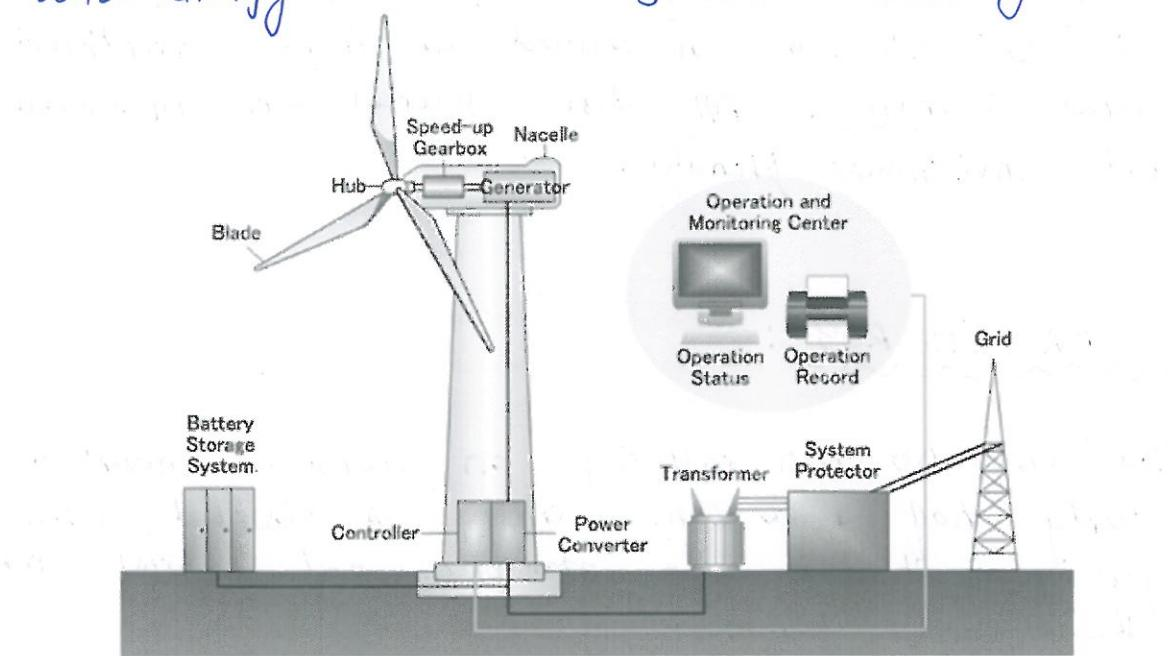
To generate electricity, rotatory motion of the windmill is used to turn the turbine of the electric generator. Large number of windmills are erected over a large area, which is known as wind energy farm. The energy output of each windmill in a farm is coupled together to get electricity on a commercial scale.
