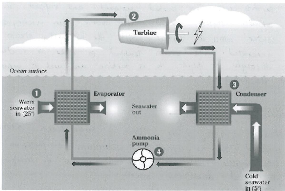
The difference in temperature at the surface of sea or ocean and water at depths up to 2 km is exploited to obtain energy in ocean-thermal-energy.
