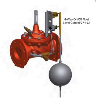
The CLA-VAL SERIES 100 On/Off Float Level Control Valve is a non-modulating valve which accurately controls the liquid level in a tank. This valve opens fully when the liquid level reaches a preset low level and closes drip tight when the liquid level reaches a high level.
