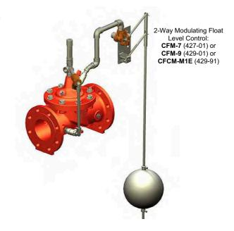
The CLA-VAL SERIES 420 Modulating Float Level Control Valve maintains a constant water level in a reservoir by compensating for variations in supply or demand. It can be installed to control the flow into or out of the reservoir by closing on rising level or opening on decreasing level.
